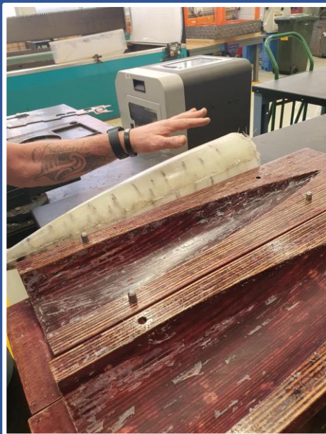
Left: Nosecone and mould after de-moulding. Above: Myself and two members of Aerostructures team after composite layup session. I gained experience with a wide variety of composite procedures during my first semester with the UQSpace Team.
